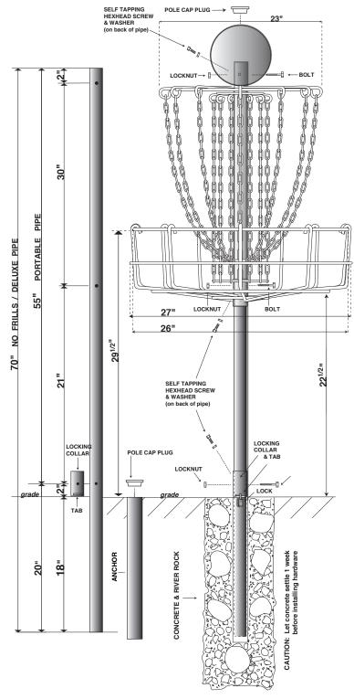
POLE (70 in.) - 1 1/2 in. I.D., 1 15/16 in. O.D. hot-dipped galvanized pipe, drilled.
